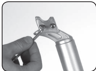
Step 6.1 Loosen the Kore I-Beam seat rail clamp with a 4mm Allen wrench.
