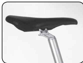
Step 6.4 Adjust the fore and aft position.
