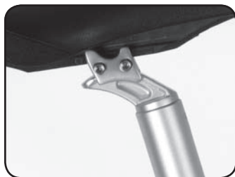
Step 6.2 Fit the saddle onto the rails.
