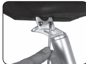
Step 6.5 Tighten the pre-greased bolts to 85 in/lbs or 9.5 NM.
